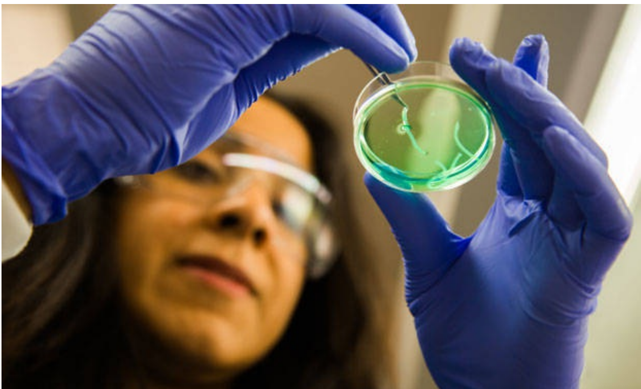
The tubular structure is created by flowing the substance through a coaxial needle source - llnl.gov
